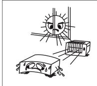
Avoid high temperatures Allow for sufficient heat dispersion when installed on a rack.
